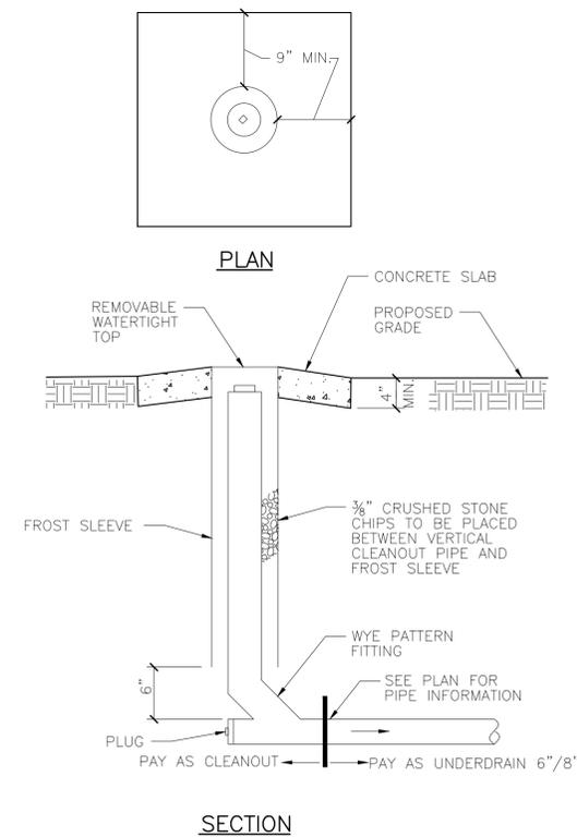
4 COLLECTOR DRAIN CLEANOUT DETAIL
