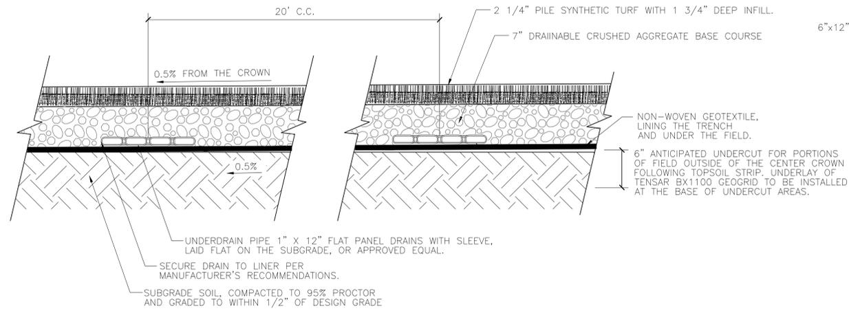
1 SYNTHETIC TURF CROSS SECTION
